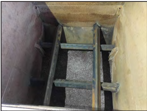
Heat Diffusers in Rock Bin & Sand Bin
